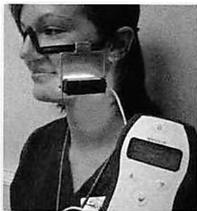
Figure 1. The OsseoPulse device consists of programmable controller and adjustable extra-oral headset and array.
